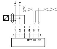
Connection with switching contact, e.g. Δp monitor
