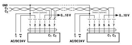
MP-Bus, supply via 3-wire connection
