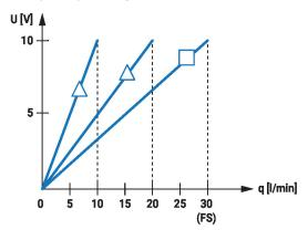
$U = Output \ voltage$   $q = Measured \ flow$   $\Delta = Alternative \ settings$   $\Box = Factory \ setting$
