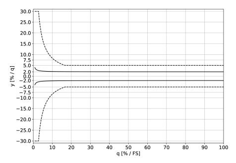
— Water ---- Water + glycol (≤60% glycol) y = Measuring accuracy q = Measured flow FS = Full scale, maximum flow
