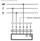
MP-Bus via 2-wire connection, local Connection with active sensor power supply
